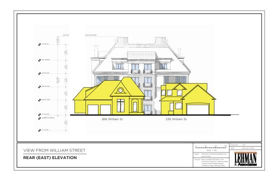
In addition I have prepared a drawing superimposing the outline of the proposed building on a plan view and front elevation of the wing of the Queen's Landing Hotel that faces Byron Street. The proposed building is approximately 66m in length and 23.5m in width. The height as calculated to the ridge of the roof is 18m. All dimensions are taken from the site plan and elevations filed with the application.
